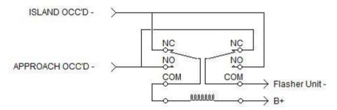
Using a Double-Pole Double-Throw relay, you can allow your crossing warning to activate when your train enters the approach circuit but deactivate once it clears the island circuit and resets when it clears the approach.
