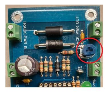
Turn the pot clockwise until the indicator on the card goes out, and then turn it back slowly just until the indicator illuminates again. You can always re-adjust the sensitivity later, but for now this should work fine. Turn off your power sources and connect your unit to the intended output devices as you desire.
