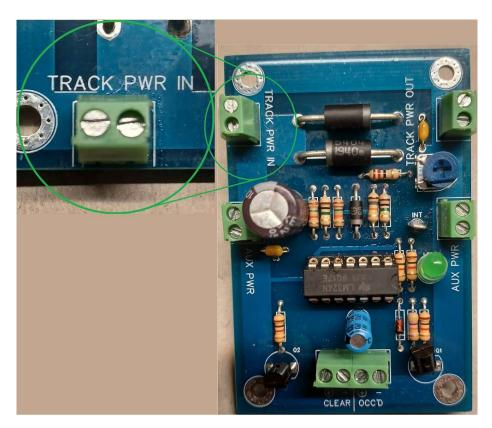
If you are using multiple detectors, it is STRONGLY recommended that you wire them all in the same general polarity with each other. Certain issues have come up with reverse polarity in the layout, even while all trains are moving in the same direction. The problem is eliminated when all the cards are aligned in the same polarity. Questions about this? Contact me for support.
