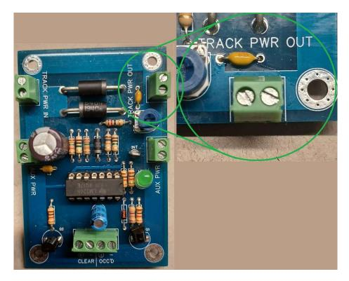
Be sure to insert your wire into each terminal and gently tighten the terminal lug with a small flat head screwdriver to finger-tightness only. DO NOT OVERTIGHTEN! For best results, it is recommended that you apply a solder tin to your wire before insertion. Alternately, you may also choose to crimp on insertion lugs at the ends of your wires.
