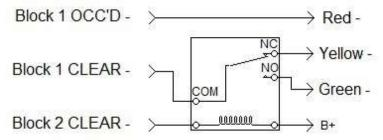
This is the diagram for using a Single Pole, Double Throw Relay to operate a 2-block system.
