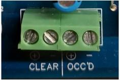
The positive output for each is only intended to drive logic inputs such as an Arduino, or other Logic Controller device. It is not advised to use this output to drive lights or motors as it may overload the unit and cause considerable damage.
