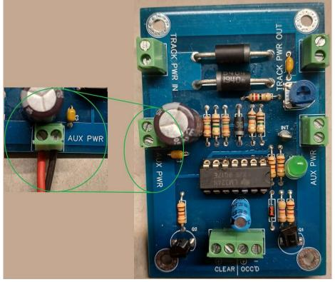
This cannot be the same power source as the track power, as it will not function. The power in to AUX power must be at least 6 volts but no more than 16 volts DC. Recommended power supply is a 12-volt DC supply.
