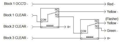
This is the diagram for using 2x SPDT relays to give the appropriate aspects for a three-block system.
